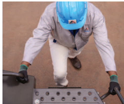
Seat belt, 3-point climbing access, and anti-slip perforated plates
